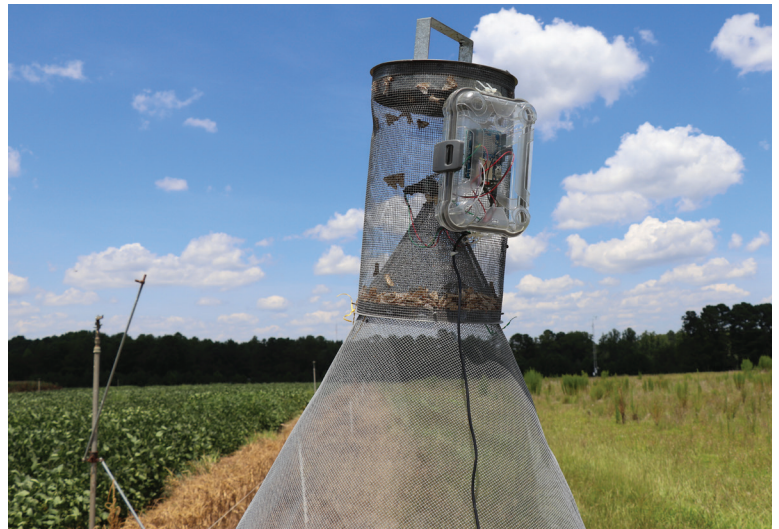
A prototype at Central Crops Research Station. The trap recorded number of moths, time moth entered the trap, temperature, and humidity.
