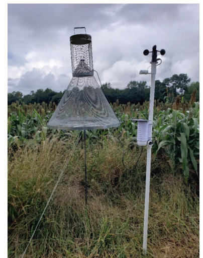
Automated corn earworm traps that can plug into mobile data networks are being tested in the field.
